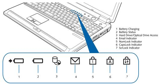
Figure 2-8. Status Indicator Panel/Volume LEDs
